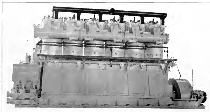
At left: The main propulsion unit of the City of San Francisco, a 6-cylinder, 4-cycle, mechanical injection, direct-reversible Western-Enterprise, 300-brake horsepower diesel engine. Below: A carload of diesel and electric machinery for the City of San Francisco leaving the Western-Enterprise shops in Los Angeles.
